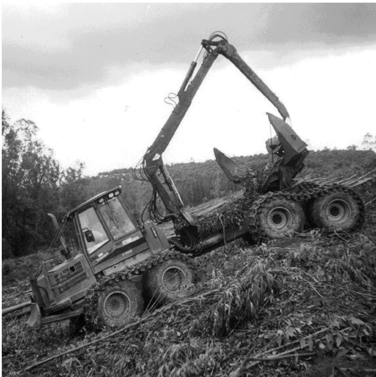
Figura 1. Trator Clambunk. (Clambunk)
